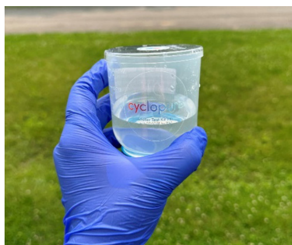
Figure 3 Cyclopure test filtering through. The sample from the HDPE bottle was poured into the Cyclopure collection cup to filter through the Dextorb pad, which extracts PFAS from the water.
