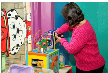
XRF testing of toys to determine if lead is present.
